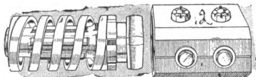
New universal joint between flywheel and gearbox of 17 H.P. Maudslay car.
